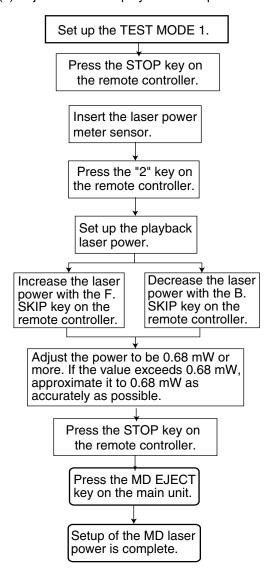
(4) Adjustment of the recording laser power
