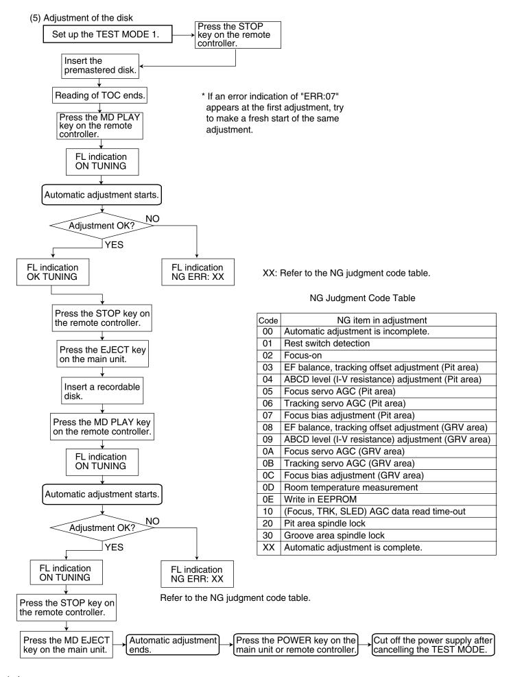
For investigating the mode in which an error occurred during the disk adjustment, freeze the set in the mode by pressing the proper key (refer to the table on the right) on the remote controller before cancelling the TEST MODE 1.
